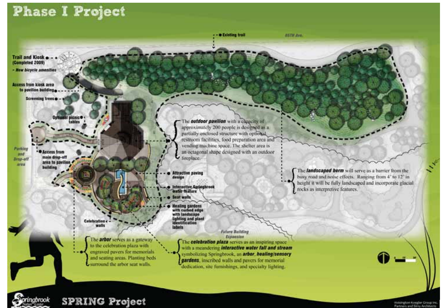
This diagram shows the first phase of the Springbrook SPRING project, the development of an outdoor pavilion and celebration plaza.
